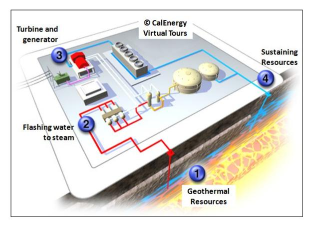
Welcome to one of CalEnergy's geothermal power plants. Unlike other power plants that reply on coal or other fossil fuels to create electricity for homes and businesses, geothermal power plants use superheated fluids from the earth's geothermal resources to generate electricity.
