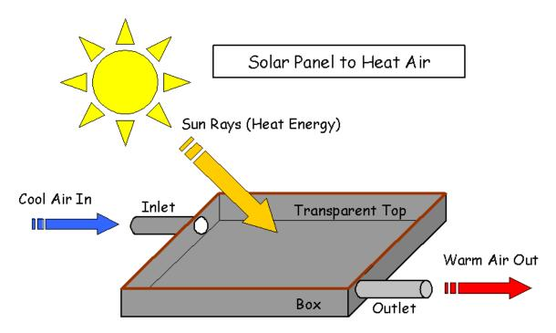
Inside the box the air is warmed by the heat energy from the sun rays. As more cool air is pushed into the box the warm air is forced out the other end of the box through the outlet pipe. The warm air can now be used to heat something like your home. Some very large systems use a solar panel on the roof of a house to heat a whole room. The warm air in that room is then blown through vents to heat the whole house.
