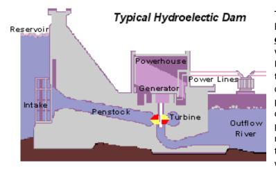
The theory is to build a dam on a large river that has a large drop in <u>elevation</u>. The dam stores lots of water behind it in the reservoir. Near the bottom of the dam wall there is the water intake. <u>Gravity</u> causes it to fall through the penstock inside the dam. At the end of the penstock there is a turbine propeller, which is turned by the moving water. The shaft from the turbine goes up into the generator, which produces the power. Power
